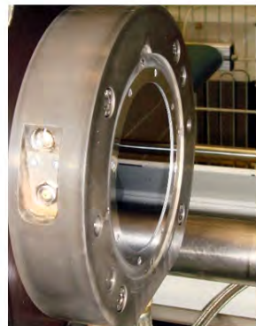
Figure 5.29: Left side: Clamping system for a 4" wafer used as insert for injection molding. Right side: Tool with ejection side of the injection mold with structured 4" silicon wafer.
