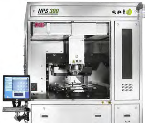
Figure 1: SET's NPS Step and Stamp machine for thermal and UV NIL used for these experiments (until 2007 SET was part of SÜSS Microtec), installed at VTT (left side), and example (right side) of a 237 consecutive thermal imprints into a 300 nm thick mr-I 7000R film (by micro resist technology GmbH ) on a 100mm Silicon wafer. Stamp size 4x4mm 2 , micrometer features with sizes of down to 2 µm and height of ~ 200nm. Stamp Temperature: 140 °C, substrate temperature 70 °C, cycle time ~ 3 minutes (without collimation and arm movements).
